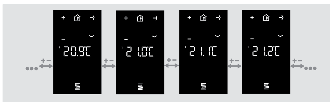
Figure 20: Setting the basic temperature / comfort temperature
