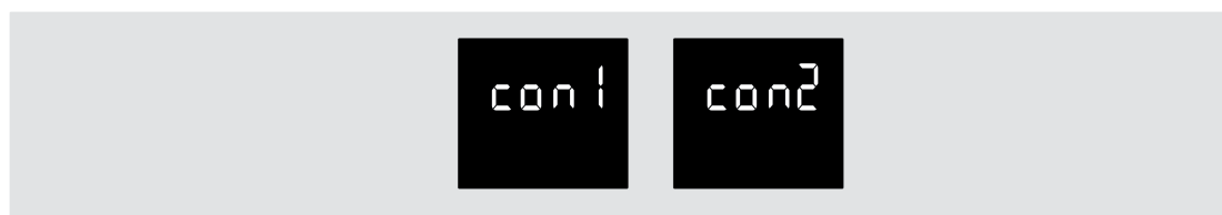
Figure 18: Display for recalling the Controller 1 and 2 submenu
