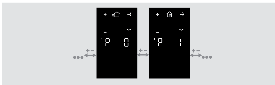
Figure 25: Setting presence mode
