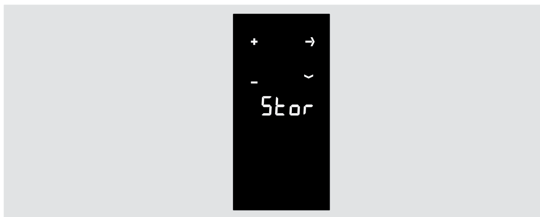
Figure 32: Exiting the menu level with saving
