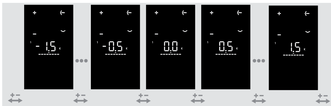
Figure 26: Setting the setpoint shift
