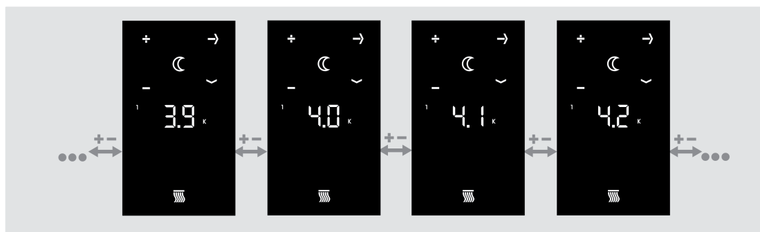
Figure 24: Setting the setpoint temperature "Raising for night mode, cooling"
