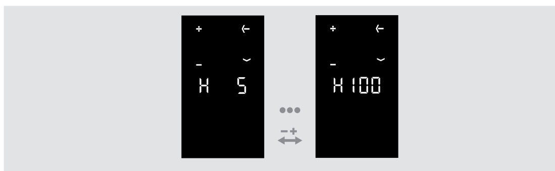
Figure 31: Setting the display brightness
