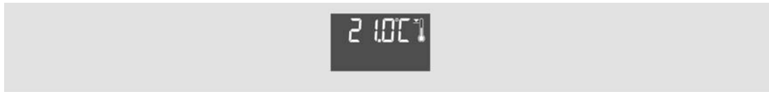
picture 21: Indication of setpoint temperature
