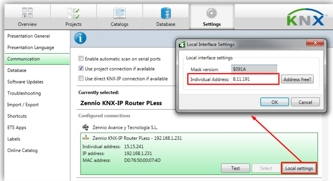
Figure 12 Configuration of the first tunneling address in ETS4.
