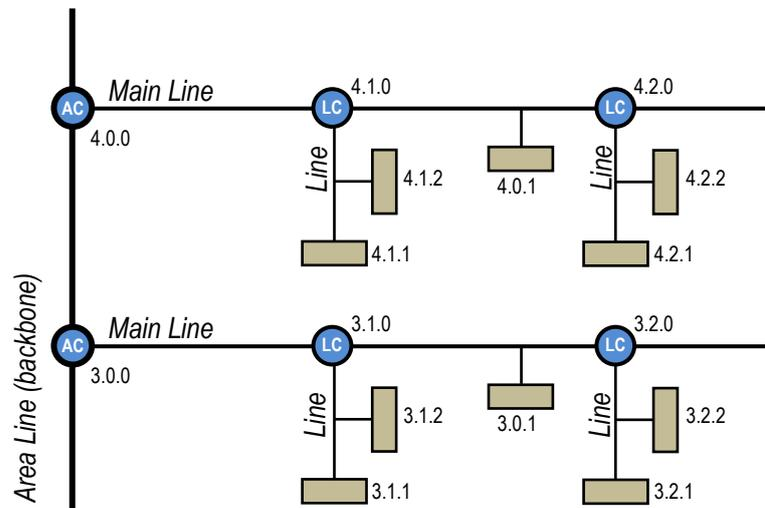
Figure 5 Line Coupling
