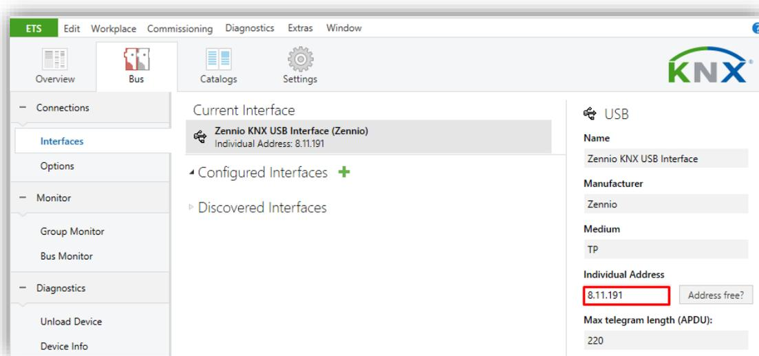
Figure 13 Configuration of the first tunneling address in ETS5.
