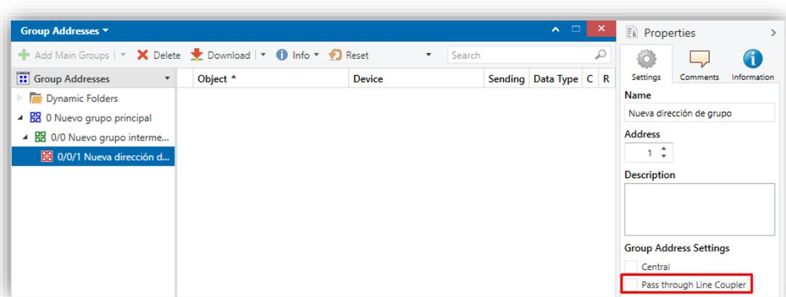
Figure 6 ETS Option to Force Passing a Group Address through the Line Coupler
