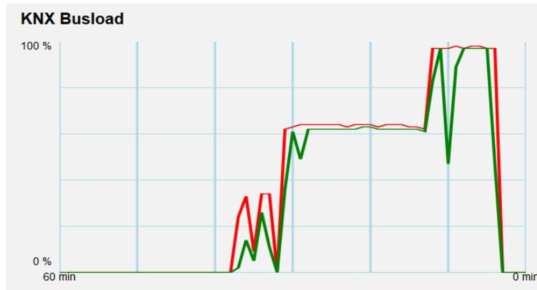
Figure 10 Web interface (KNX bus load)
