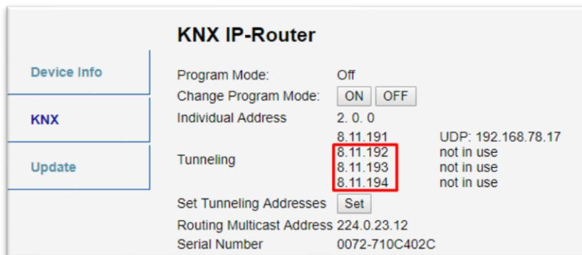
Figure 11 Set tunneling addresses in web interface.
