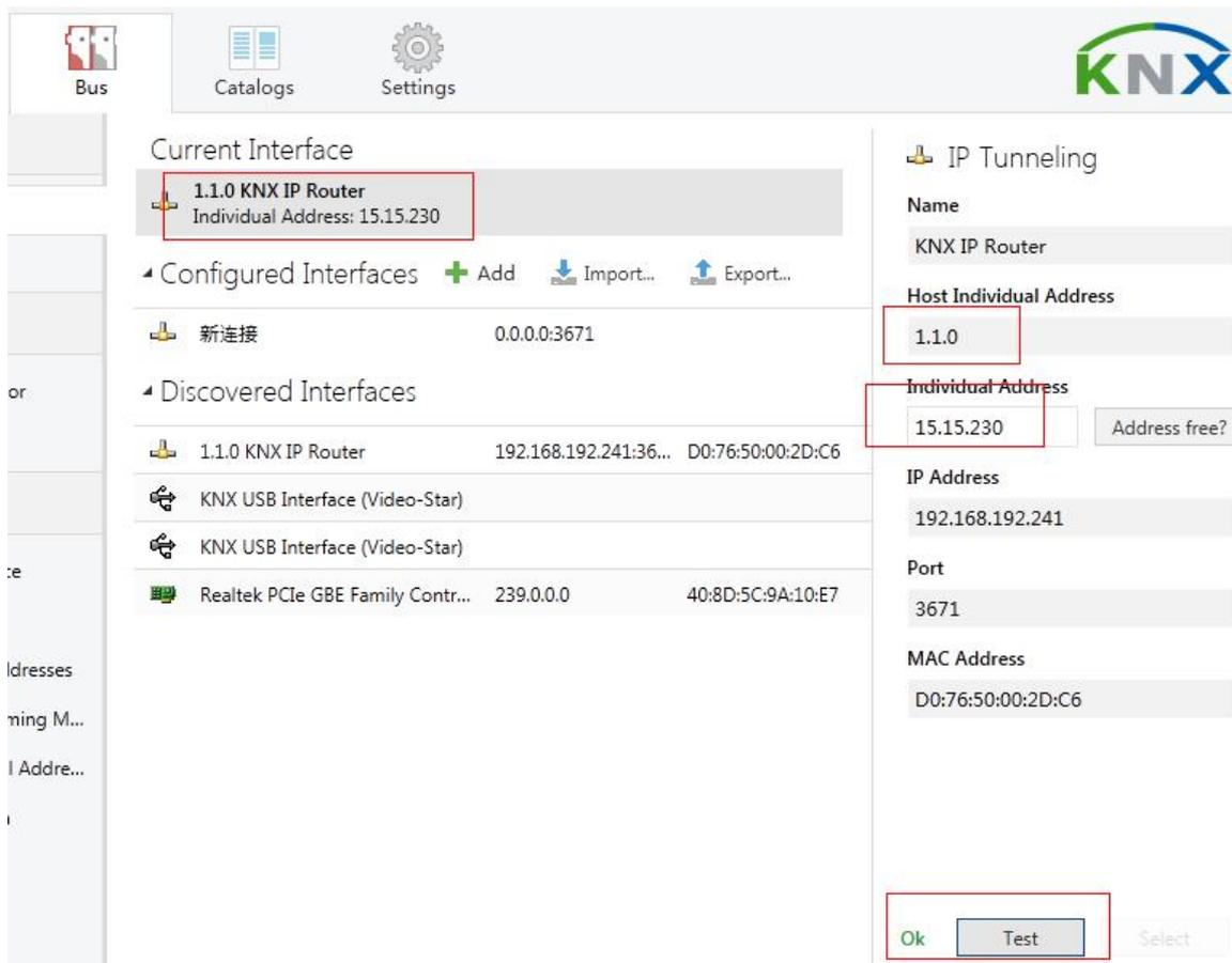
Fig. 5.10: First Additional Physical Address (First Tunneling Address)
