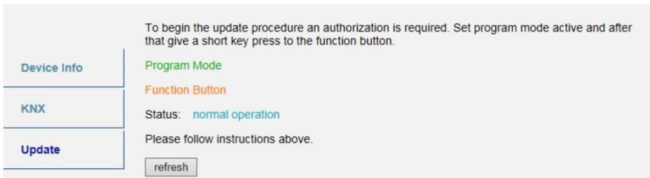
Fig. 5.6: Update Tab and activated Programming Mode
