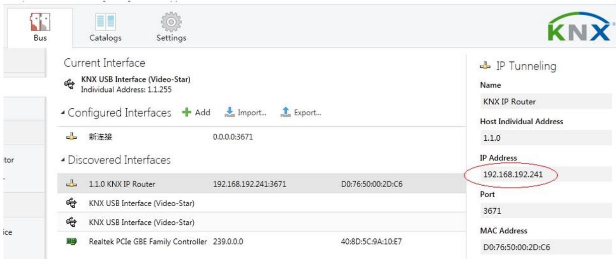
Fig. 5.2: Identifying IP address with ETS
