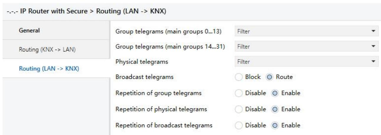
Fig. 5.3 Parameter window "Routing(LAN->KNX)"
