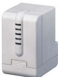
The Electromotor Valve Drive ST/K 1.1 is a proportional valve drive for controlling heating valves via the ABB i-bus® EIB. The valve drive is mounted on thermostat valve bases. The control is carried out via a continuous EIB / KNX room thermostat.
